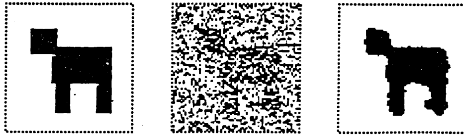
Figure 7.9 Image Restoration Based on Markov Random Field Model, from Marroquin [1985].
