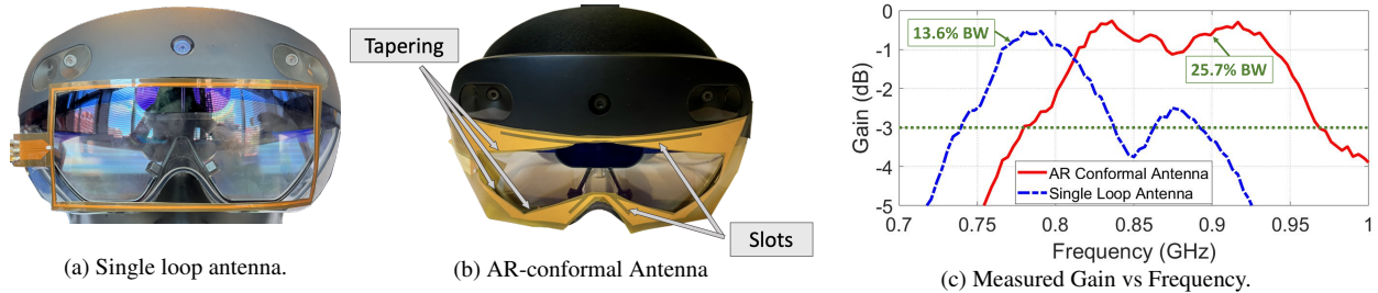
Figure 2: Conformal Antenna Design. (a) Fabricated single-loop antenna mounted on the headset (dimensions 122 \times 51 mm). (b) Fabricated conformal antenna (dimensions 165 \times 64 mm). (c) These plots show the measured gains of the single loop (blue) and AR conformal (red) antennas vs frequency while mounted on the headset and worn by the user. The horizontal green line is used to highlight the 3-dB bandwidth.
